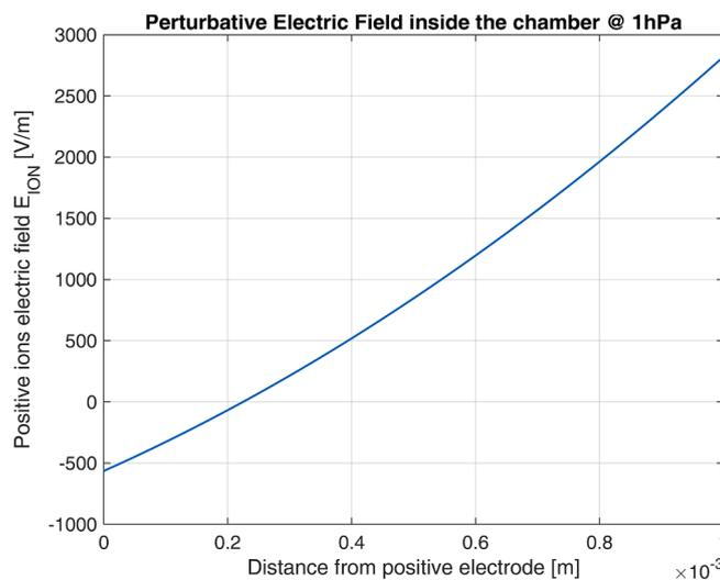
Fig. C2. Perturbative Electric Field inside the chamber.
