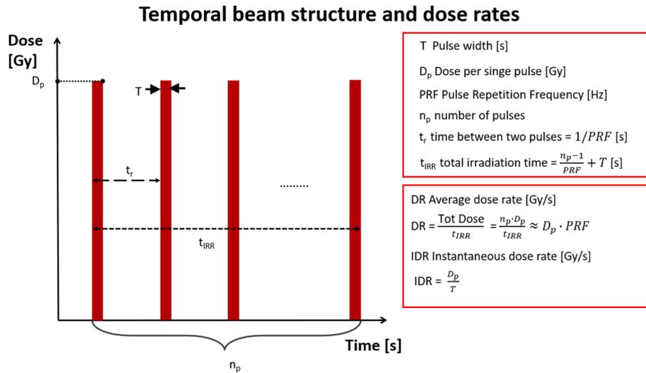
Fig. 1. Temporal beam structure and dose rate definition.
